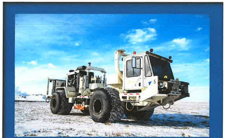
Vibroseis trucks drive across the landscape, stopping to generate vibrations every 110 feet along straight paths throughout the study area, avoiding buildings and infrastructure.
