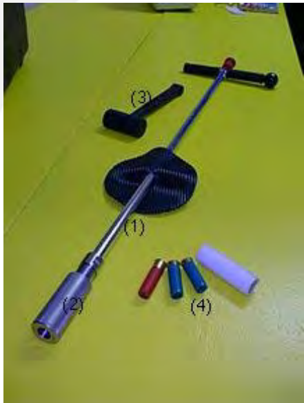
Betsy seisgun (1) with plastic splatter guard, shell holder(2), hammer(3) and shells of various sizes
