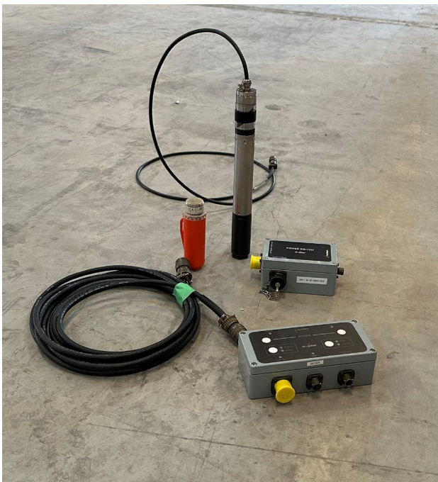
Figure 1: (Left) 2023 Next Gen Beta version of PinPoint system, weighing less than 1 kg, with STRYDE node for scale. (Right), the front page of the US Patent granted to Allan Châtenay, the inventor of the system.
