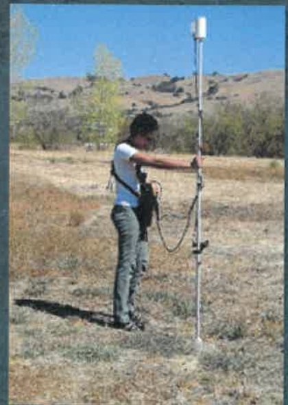
Example of a magnetic survey: a magnetometer measurement in progress.
