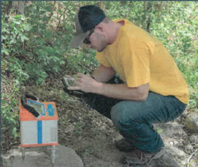
Technicians carry battery-operated gravity survey instruments to collect readings every 165 feet along paths throughout the study area.
