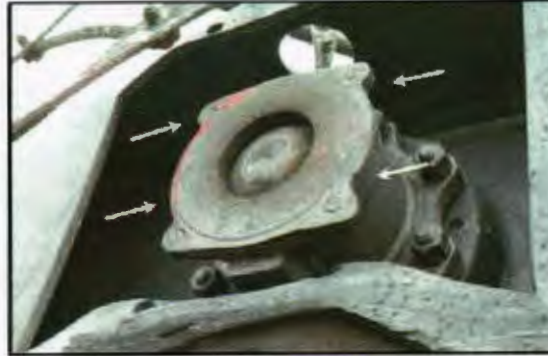
Photo 26. Bottom outlet valve with sheared-off nozzle
