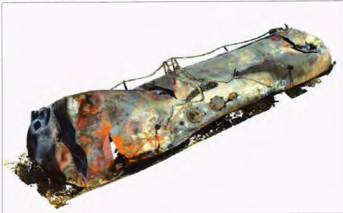
Photo 16. 3D laser scan of badly deformed tank
