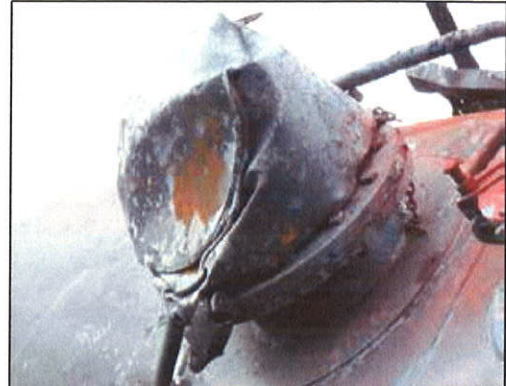
Photo 22. Hinged housing for tank car fittings
