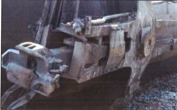
Photo 17. Complete stub sill
