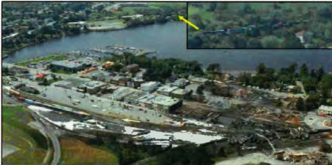
Photo 6. Location of the locomotive consist (Mile 116.41 of the Moosehead Subdivision) in relation to the derailment site. The white arrows denote the route of the locomotive consist, which followed the main track.
