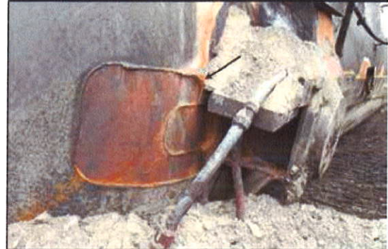
Photo 18. Damaged stub sill
