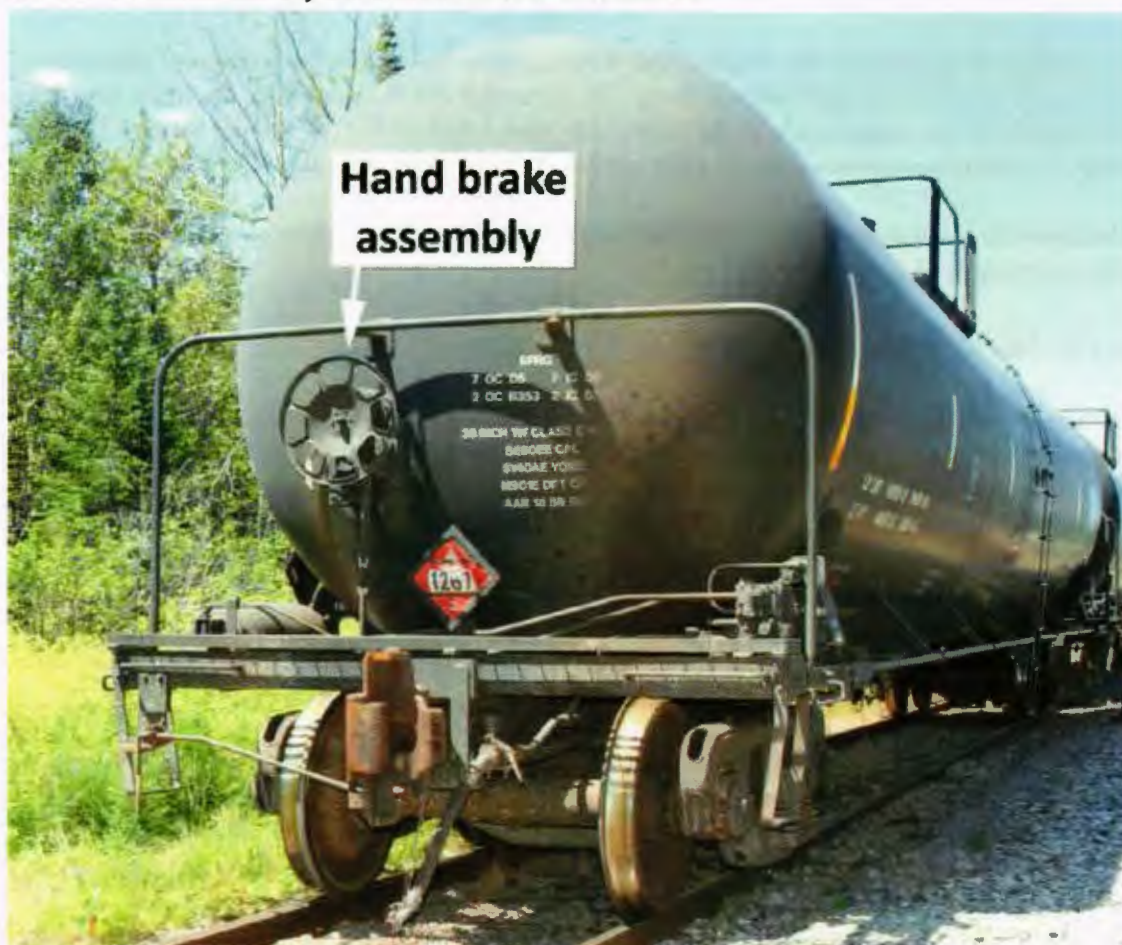
Photo 9. Hand brake assembly and wheel at the B-end of a tank car
