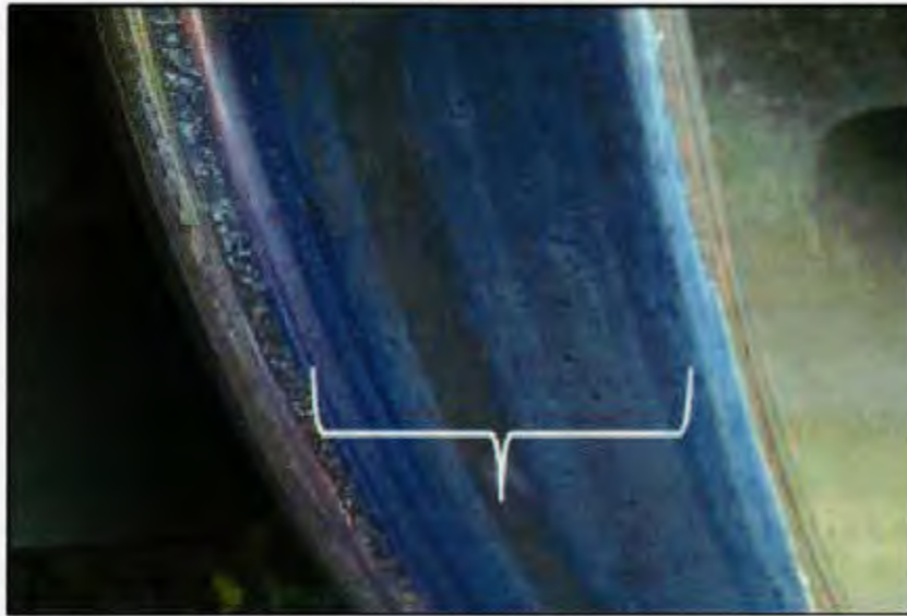
Photo 12. Blueing of locomotive wheel due to heat
