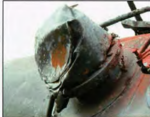
Photo 22. Hinged housing for tank car fittings
