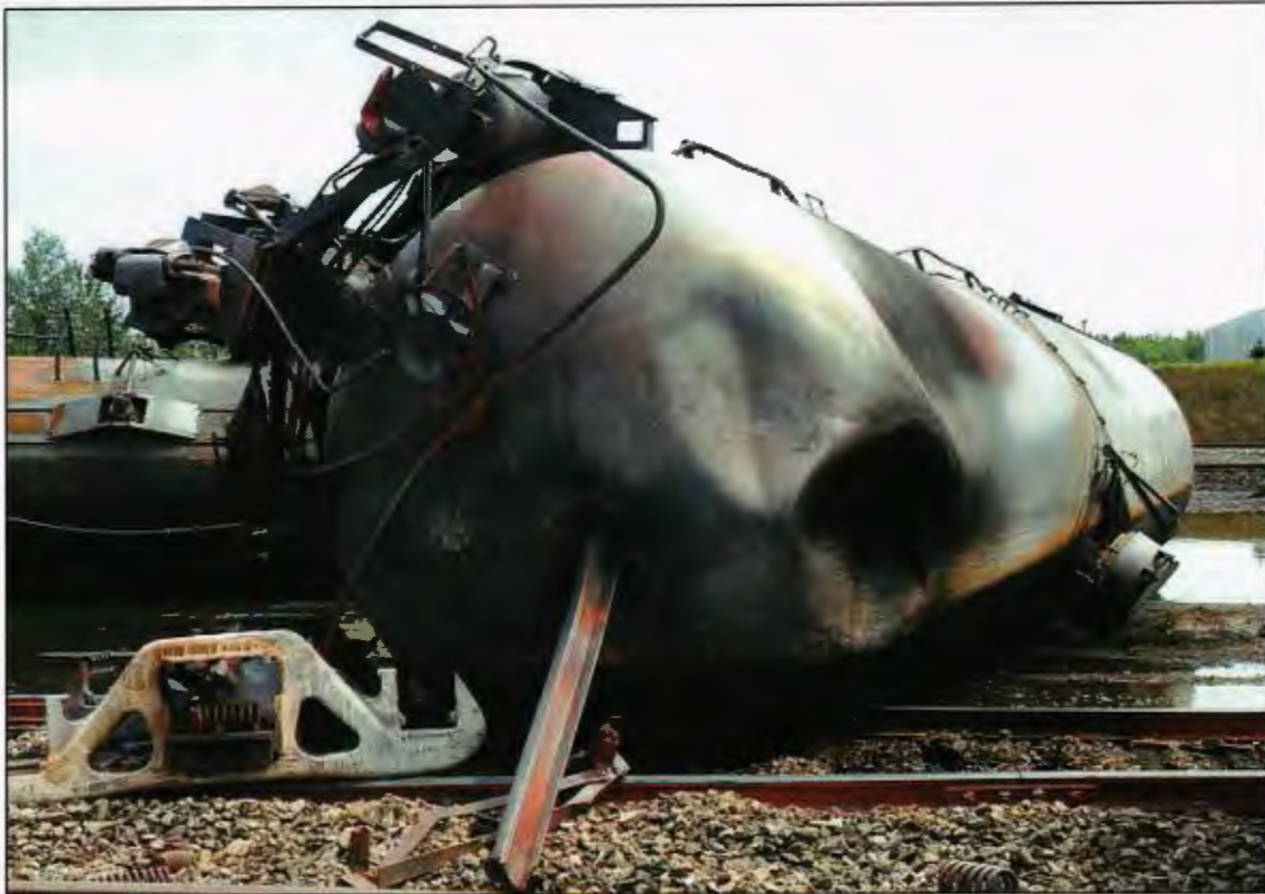
Photo 20. Head puncture due to rail impact
