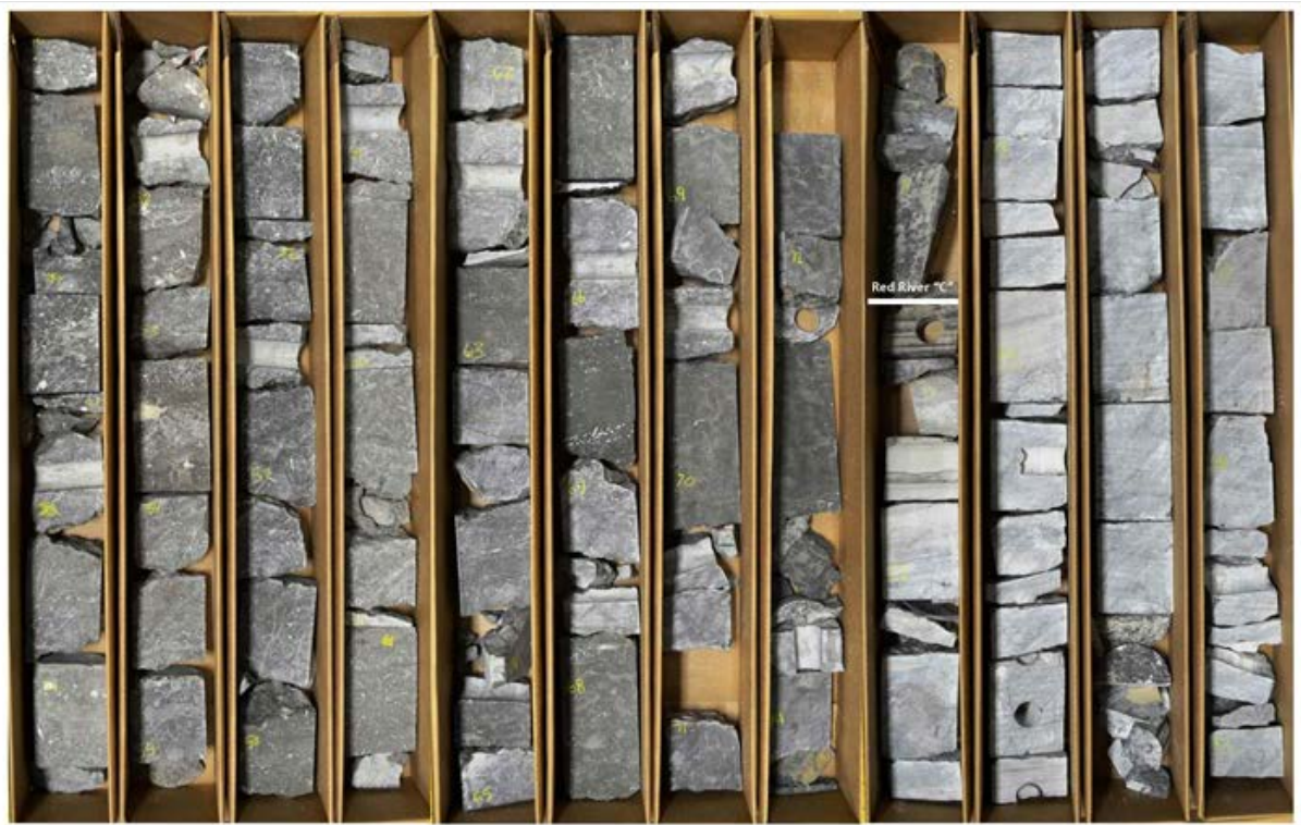
Thirty-six feet of Red River core (10,149 – 10,187 feet) from the Urlacher State Unit #1 in Hettinger County. The base of the Red River “C” is much more organic rich than the underlying limestone.
