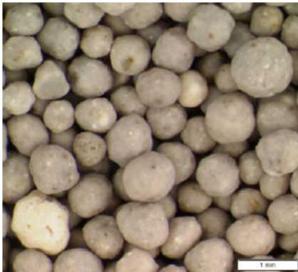
Photomicrograph of ceramic proppant from a batch that was used in a Bakken well in North Dakota. This proppant was manufactured in China.
