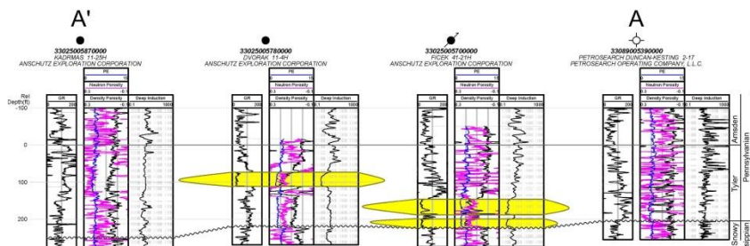
Figure 4. Cross-section extending from A to A' along the light blue line in Figure 5. The section 2-17 (#14675 on Figure 5) corresponds to the point labeled A. Conventional sandstone reservoirs of the Tyler Formation.
