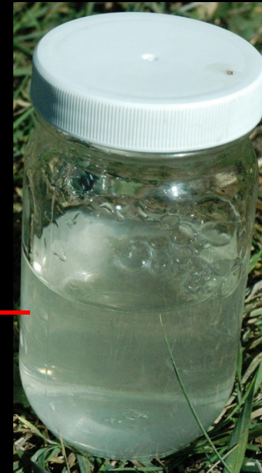
Methane bubbles in a groundwater sample recently obtained from a private well southwest of Harwood in Cass County (large star on map).
