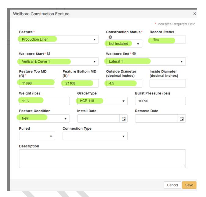
The above info is based off the operator's Casing Design Parameters as noted after this section.
