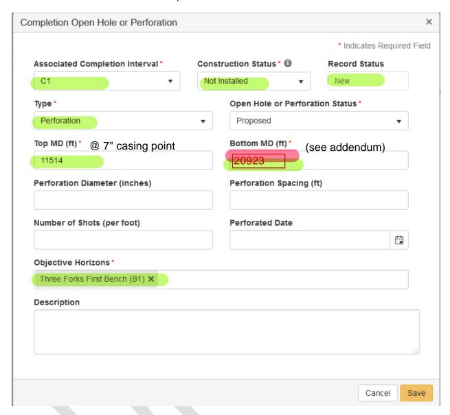
Note: Enter the following info if it is known at the time of permitting: Perforation Diameter, Perforation Spacing & Number of shots. The information displayed is the minimum we would allow. We would prefer that the operator indicate the top & bottom MD perforations. This information should be found on the Bakken Completion Schematic.
