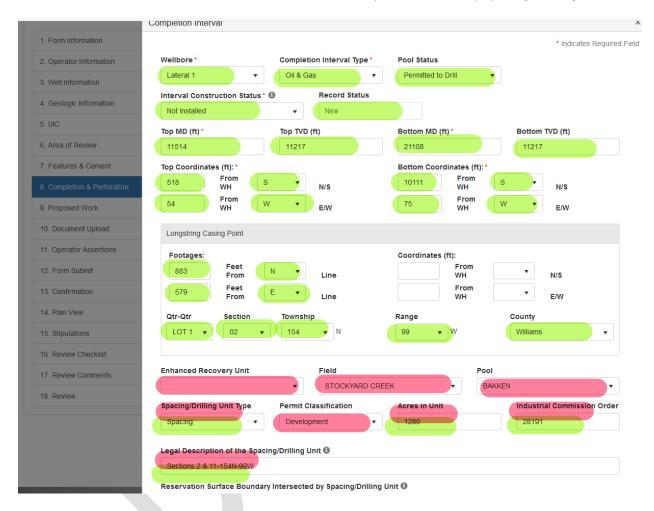
Typical "Bakken" single laterals: 7" (production) casing point will be the "top" of the completion interval, and bottom will be dependent upon the type toe isolation.
