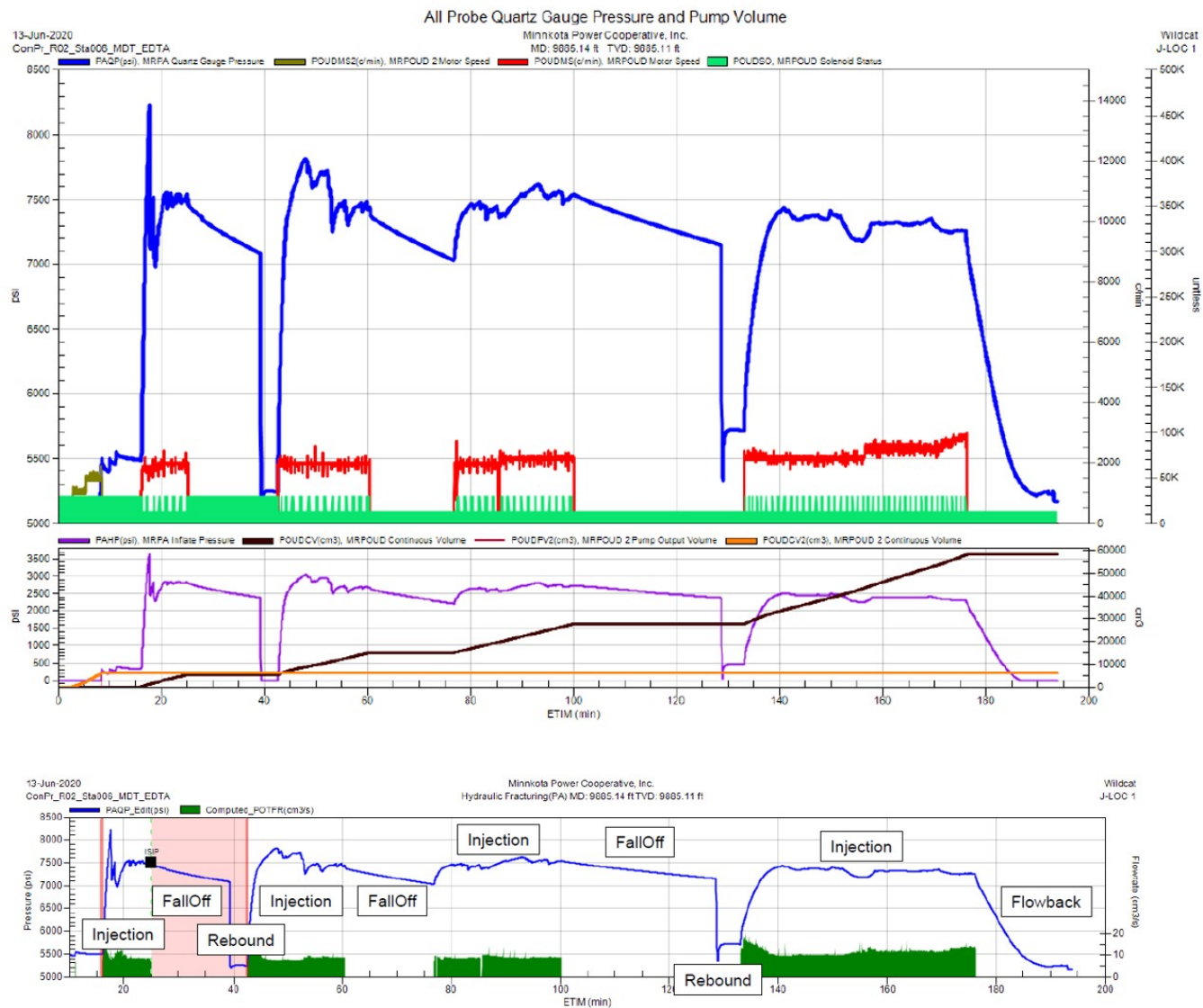
Figure 2-16. J-LOC1 Deadwood Formation MDT microfracture in situ stress pump cycle graph at 9,885.1 ft.
