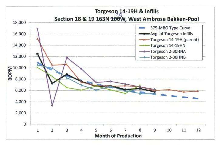
Early infill well production compared to parent-well production in Sections 18 & 19, 163N 100W. The Torgeson wells have an average inter-well distance of approximately 1,100'. The average performance of the infills exceeds the 375 MBO-type curve, which indicates that wells spaced 1,100 - 1,400' apart (320-acre spacing) should be economic.
