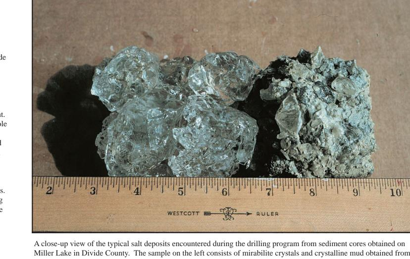
a depth of 22 to 22.8 feet within Hole No. 1 from Miller Lake. Workers have commented that drilling conditions were very difficult in the individual salt layers and stabilization of the salt layers was within question due to local influences
