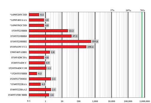
Figure 1. Graph depicting the relative relationship and absolute maximum values of flame-ionization detector (FID) instrument responses from selected wells in Grand Forks County. FID results for each well are presented in order of field screening occurrence from top to bottom. Values shown are those reported from the ground-water/air interface (GWI) (as CH4 in ppm). The concentration of methane typical in commercial natural gas is highlighted by the vertical green line at 70%.
