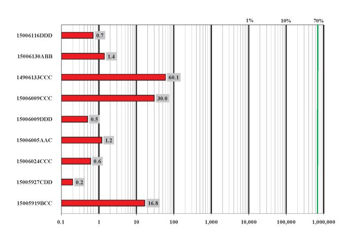
Figure 1. Graph depicting the relative relationship and absolute maximum values of flame-ionization detector (FID) instrument responses from selected wells in Nelson County. FID results for each well are presented in order of field screening occurrence from top to bottom. Values shown are those reported from the ground-water/air interface (GWI) (as CH4 in ppm). The concentration of methane typical in commercial natural gas is highlighted by the vertical green line at 70%.
