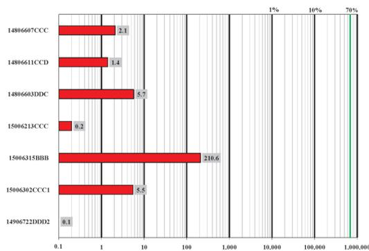
Figure 1. Graph depicting the relative relationship and absolute maximum values of flame-ionization detector (FID) instrument responses from selected wells in Eddy County. FID results for each well are presented in order of field screening occurrence from top to bottom. Values shown are those reported from the ground-water/air interface (GWI) (as CH<sub>4</sub> in ppm). The concentration of methane typical in commercial natural gas is highlighted by the vertical green line at 70%.
