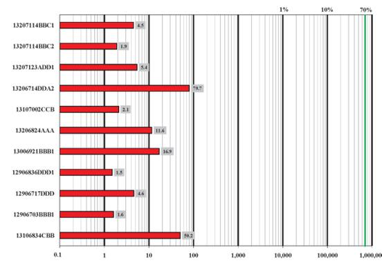
Figure 1. Graph depicting the relative relationship and absolute maximum values of flame-ionization detector (FID) instrument responses from selected wells in McIntosh County. FID results for each well are presented in order of field screening occurrence from top to bottom. Values shown are those reported from the ground-water/air interface (GWI) (as CH<sub>4</sub> in ppm). The concentration of methane typical in commercial natural gas is highlighted by the vertical green line at 70%.
