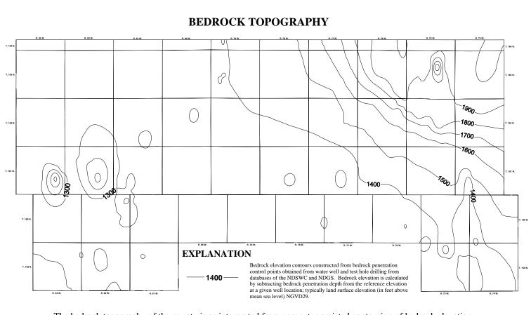
The bedrock topography of the county is as interpreted from computer-assisted contouring of bedrock elevation values determined for the county. Structure contours delineate area of highest bedrock elevations in the northeast portion of the county, in the vicinity of the Turtle Mountains, and slope away from this feature towards the southwest into the relatively flat central portion of the county. Local structural relief is present in the western portion of the county.
