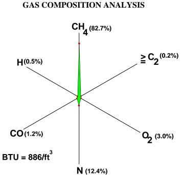
Star diagram of gas composition analysis from shallow gas occurrence in well located on the Parker Farm (Barry, 1908) in T.161N., R.80W.
