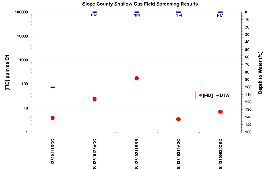
Figure 21. Shallow gas field screening results in Slope County. FID response [FID] in ppm as C1 is plotted on the logarithmic scale on the primary y-axis. Depth to water measurements are plotted on the secondary y-axis. NM = Not Measured. S = Stock Well.
