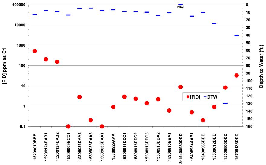
Figure 26. Shallow gas field screening results in Mountrail County. FID response [FID] in ppm as C1 is plotted on the logarithmic scale on the primary y-axis. Depth to water measurements are plotted on the secondary y-axis. NM = Not Measured. S = Stock Well.
