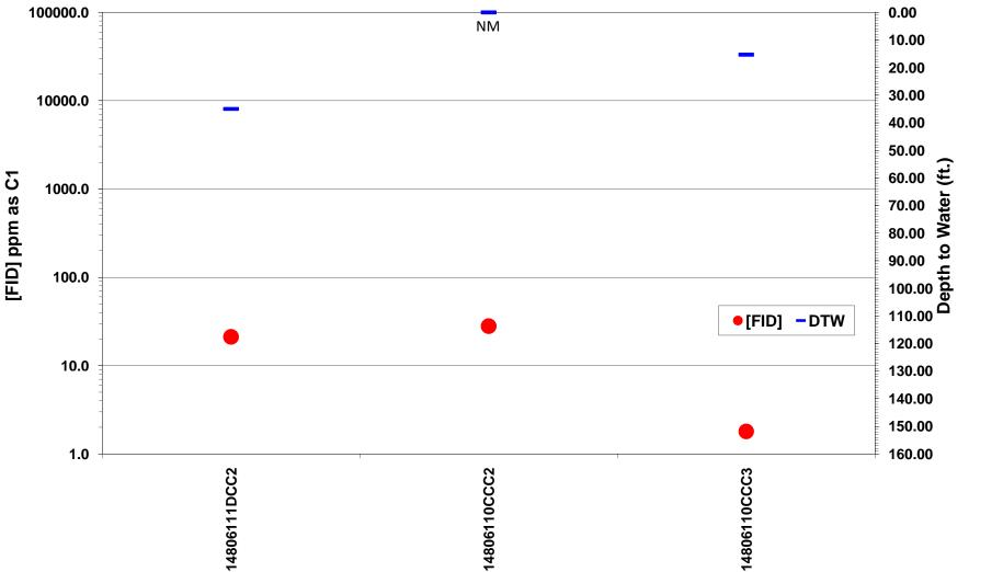
Figure 14. Shallow gas field screening results in Oliver County. FID response [FID] in ppm as C1 is plotted on the logarithmic scale on the primary y-axis. Depth to water measurements are plotted on the secondary y-axis. NM = Not Measured.
