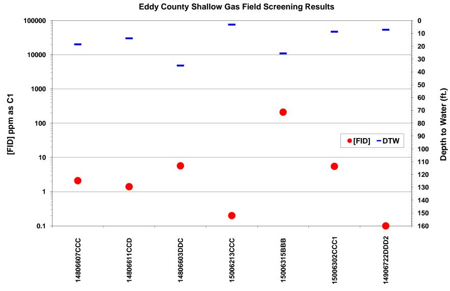
Figure 37. Shallow gas field screening results in Eddy County. FID response [FID] in ppm as C1 is plotted on the logarithmic scale on the primary y-axis. Depth to water measurements are plotted on the secondary y-axis.
