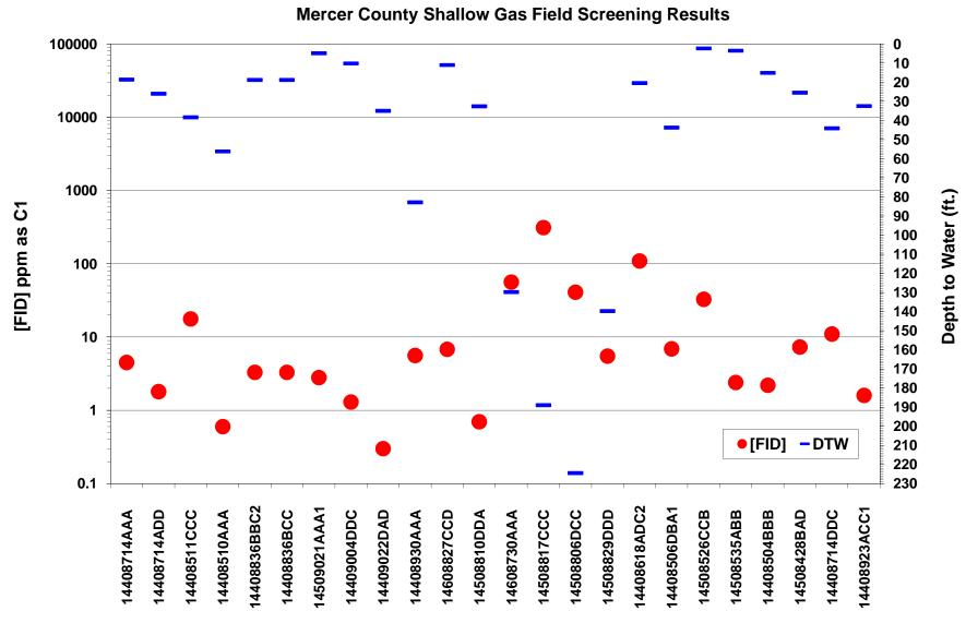
Figure 15. Shallow gas field screening results in Mercer County. FID response [FID] in ppm as C1 is plotted on the logarithmic scale on the primary y-axis. Depth to water measurements are plotted on the secondary y-axis.
