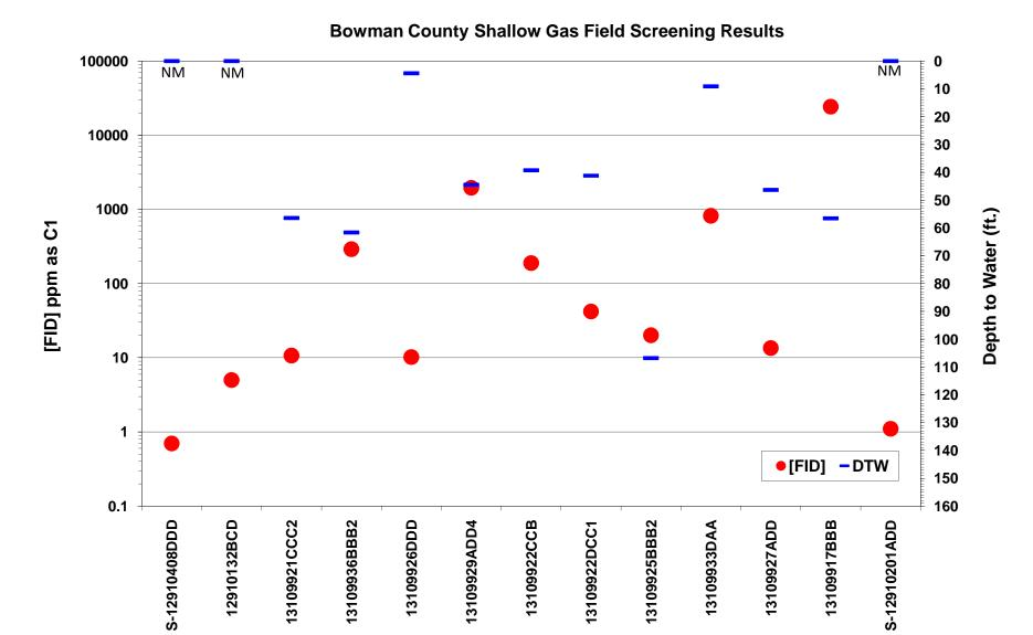
Figure 16. Shallow gas field screening results in Bowman County. FID response [FID] in ppm as C1 is plotted on the logarithmic scale on the primary y-axis. Depth to water measurements are plotted on the secondary y-axis. NM = Not Measured. S = Stock Well.
