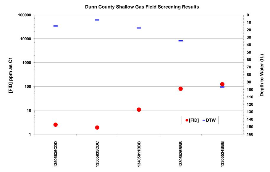
Figure 18. Shallow gas field screening results in Dunn County. FID response [FID] in ppm as C1 is plotted on the logarithmic scale on the primary y-axis. Depth to water measurements are plotted on the secondary y-axis.
