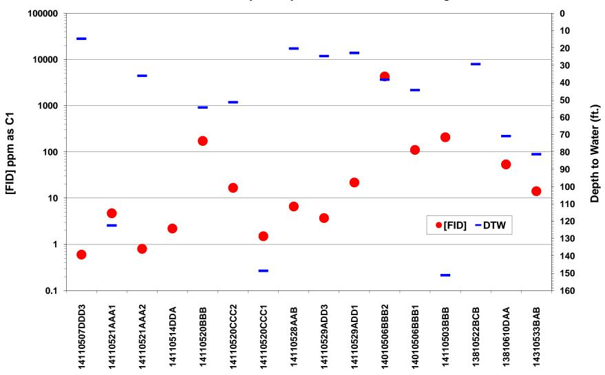
Figure 24. Shallow gas field screening results in Golden Valley County. FID response [FID] in ppm as C1 is plotted on the logarithmic scale on the primary y-axis. Depth to water measurements are plotted on the secondary y-axis.
