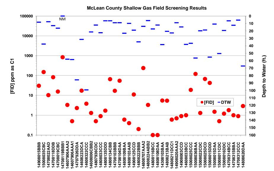
Figure 22. Shallow gas field screening results in McLean County. FID response [FID] in ppm as C1 is plotted on the logarithmic scale on the primary y-axis. Depth to water measurements are plotted on the secondary y-axis. NM = Not Measured.
