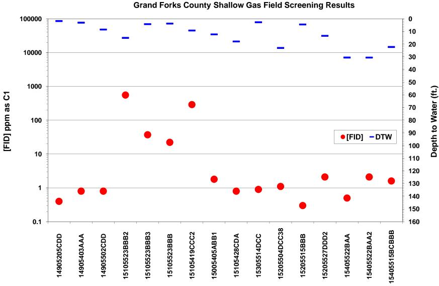
Figure 42. Shallow gas field screening results in Grand Forks County. FID response [FID] in ppm as C1 is plotted on the logarithmic scale on the primary yaxis. Depth to water measurements are plotted on the secondary y-axis.
