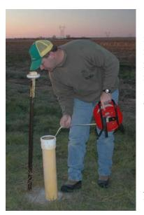
Depth to water measurements (in feet) were taken at each well field screened where a positive FID instrument response was recorded. A total depth of well measurement was also consecutively collected, when required, in order to identify individual wells within well nests that were not readily identifiable in the field. All ground-water level measurements were collected with an electronic well tape during field screening.
