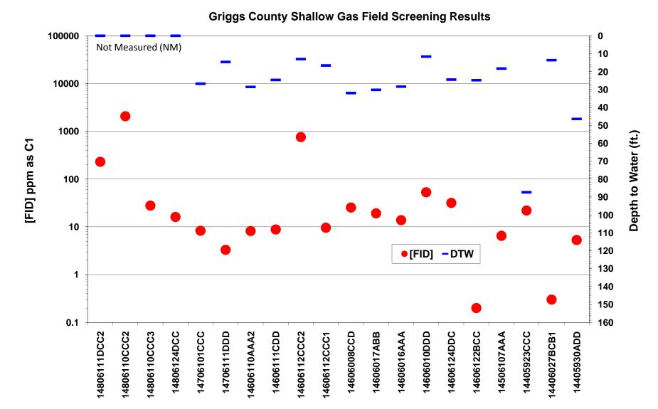
Figure 13. Shallow gas field screening results in Griggs County. FID response [FID] in ppm as C1 is plotted on the logarithmic scale on the primary y-axis. Depth to water measurements are plotted on the secondary y-axis.
