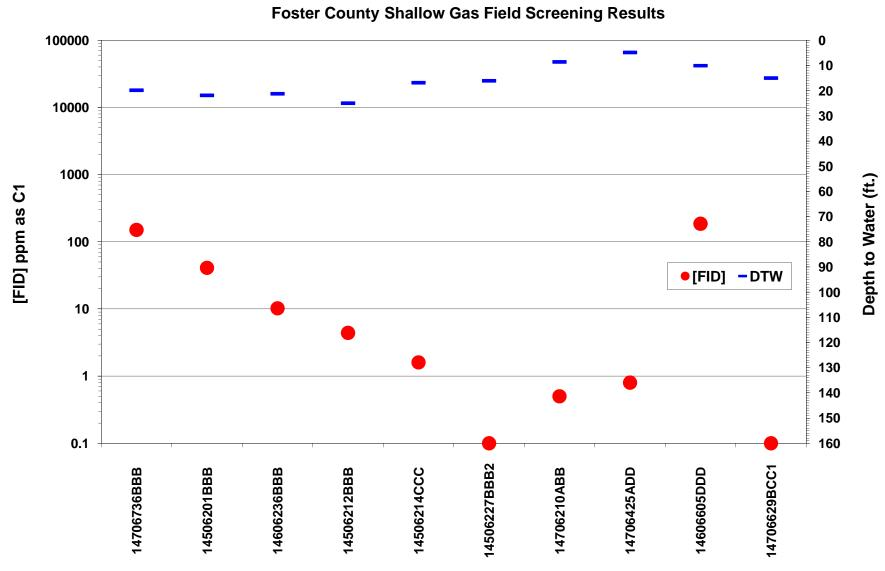
Figure 38. Shallow gas field screening results in Foster County. FID response [FID] in ppm as C1 is plotted on the logarithmic scale on the primary y-axis. Depth to water measurements are plotted on the secondary y-axis.
