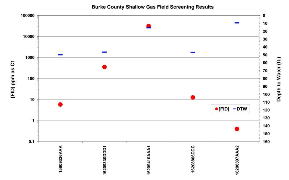
Figure 27. Shallow gas field screening results in Burke County. FID response [FID] in ppm as C1 is plotted on the logarithmic scale on the primary y-axis. Depth to water measurements are plotted on the secondary y-axis.
