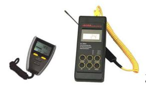
Figure 6. Field instrumentation used for the collection of atmospheric pressure and temperature.
