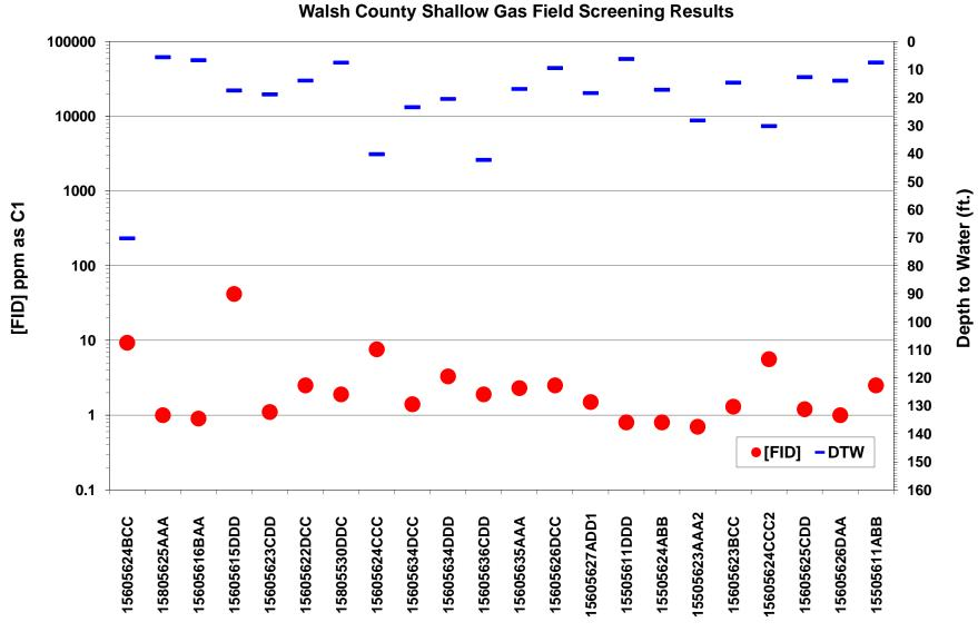
Figure 43. Shallow gas field screening results in Walsh County. FID response [FID] in ppm as C1 is plotted on the logarithmic scale on the primary y-axis. Depth to water measurements are plotted on the secondary y-axis.
