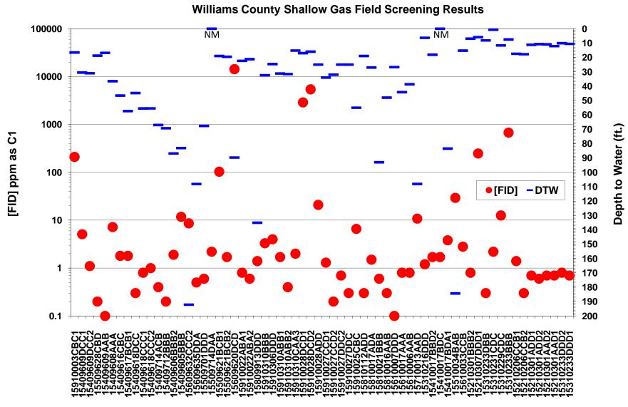
Figure 36. Shallow gas field screening results in Williams County. FID response [FID] in ppm as C1 is plotted on the logarithmic scale on the primary y-axis. Depth to water measurements are plotted on the secondary y-axis. NM = Not Measured.
