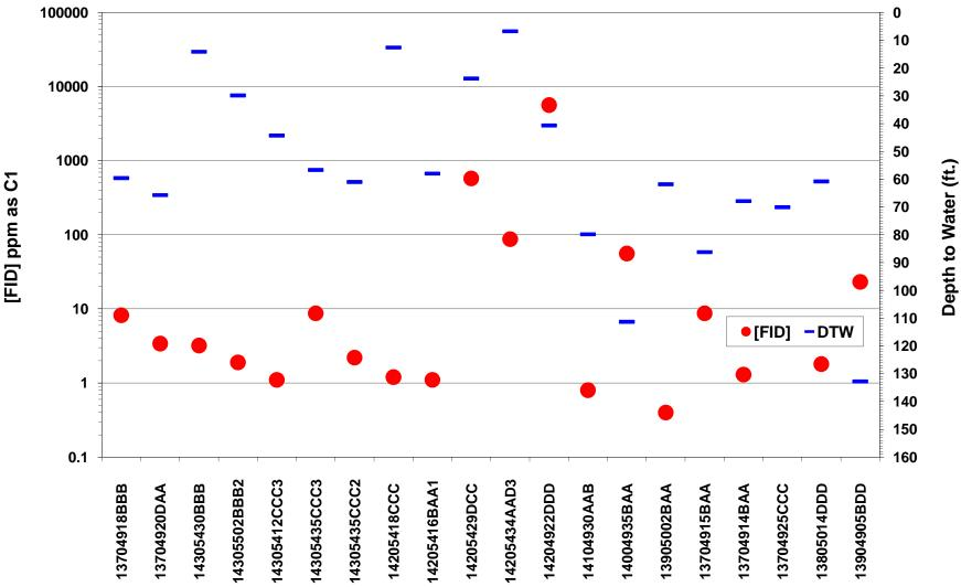
Figure 33. Shallow gas field screening results in Cass County. FID response [FID] in ppm as C1 is plotted on the logarithmic scale on the primary y-axis. Depth to water measurements are plotted on the secondary y-axis.
