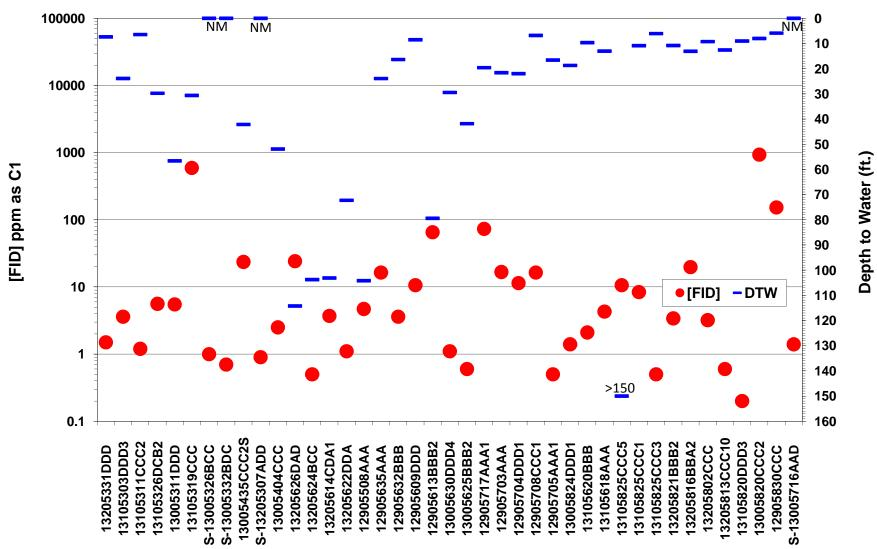
Figure 30. Shallow gas field screening results in Sargent County. FID response [FID] in ppm as C1 is plotted on the logarithmic scale on the primary y-axis. Depth to water measurements are plotted on the secondary y-axis. NM = Not Measured. S = Stock Well.
