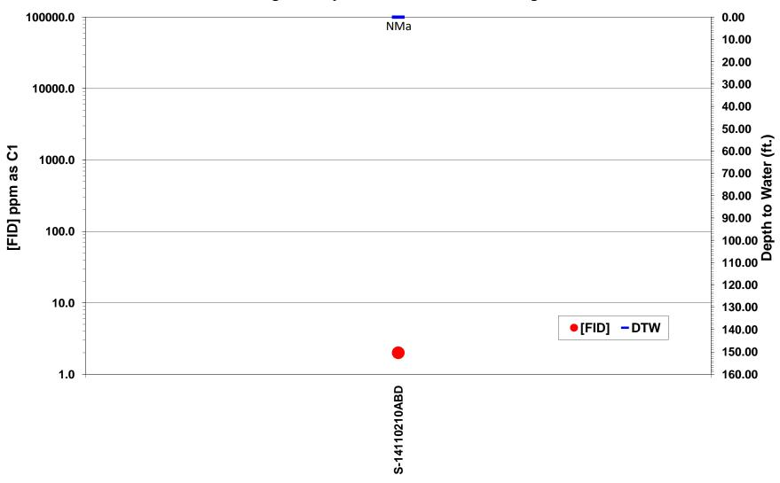
Figure 20. Shallow gas field screening results in Billings County. FID response [FID] in ppm as C1 is plotted on the logarithmic scale on the primary y-axis. Depth to water measurements are plotted on the secondary y-axis. NM = Not Measured. S = Stock Well. a = artesian well.
