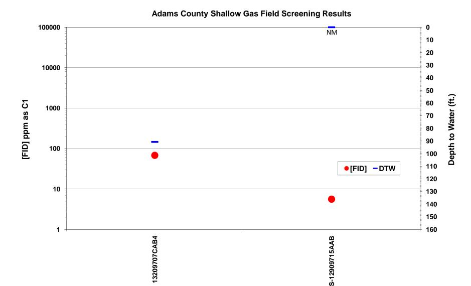
Figure 25. Shallow gas field screening results in Adams County. FID response [FID] in ppm as C1 is plotted on the logarithmic scale on the primary y-axis. Depth to water measurements are plotted on the secondary y-axis. NM = Not Measured. S = Stock Well.
