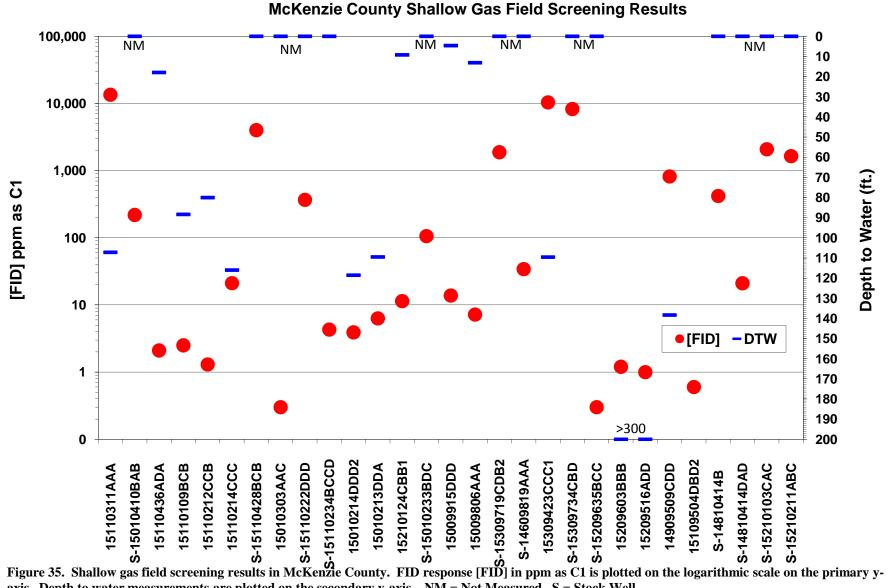
axis. Depth to water measurements are plotted on the secondary y-axis. NM = Not Measured. S = Stock Well.
