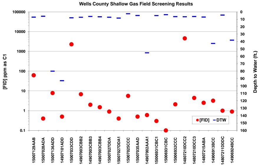
Figure 34. Shallow gas field screening results in Wells County. FID response [FID] in ppm as C1 is plotted on the logarithmic scale on the primary y-axis. Depth to water measurements are plotted on the secondary y-axis.
