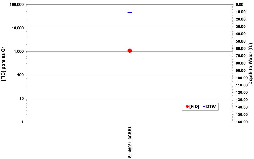
Figure 12. Shallow gas field screening results in Traill County. FID response [FID] in ppm as C1 is plotted on the logarithmic scale on the primary y-axis. Depth to water measurements are plotted on the secondary y-axis.
