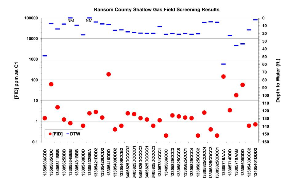
Figure 17. Shallow gas field screening results in Ransom County. FID response [FID] in ppm as C1 is plotted on the logarithmic scale on the primary y-axis. Depth to water measurements are plotted on the secondary y-axis. NM = Not Measured.
