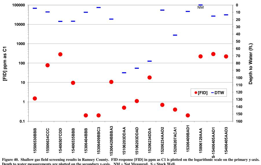
Depth to water measurements are plotted on the secondary y-axis. NM = Not Measured. S = Stock Well.
