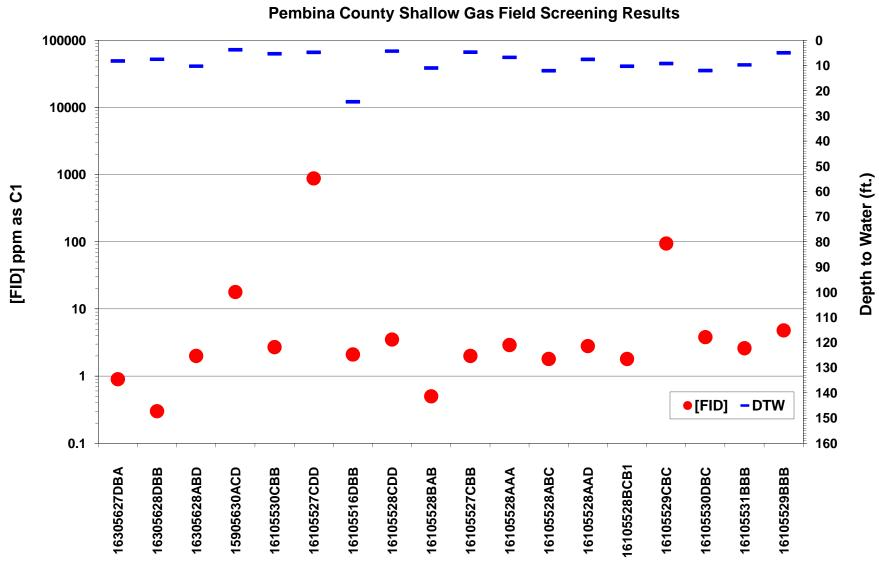
Figure 44. Shallow gas field screening results in Pembina County. FID response [FID] in ppm as C1 is plotted on the logarithmic scale on the primary y-axis. Depth to water measurements are plotted on the secondary y-axis.
