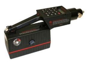
Figure 2. Photovac portable Flame Ionization Detector (FID) used in this investigation.
