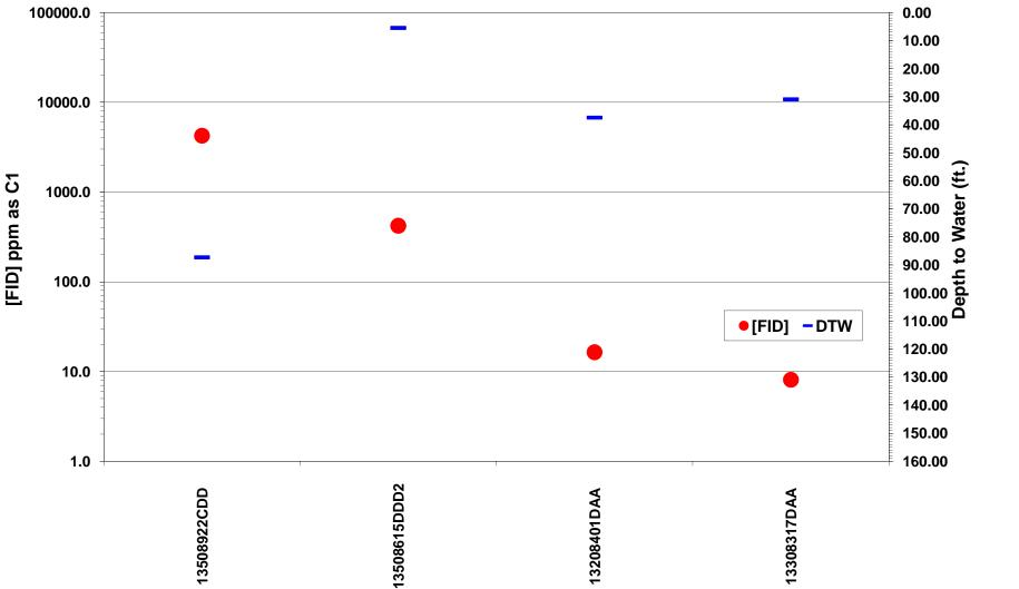
Figure 28. Shallow gas field screening results in Grant County. FID response [FID] in ppm as C1 is plotted on the logarithmic scale on the primary y-axis. Depth to water measurements are plotted on the secondary y-axis.
