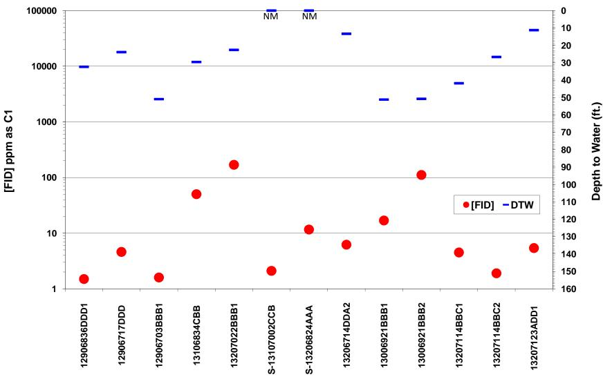
Figure 32. Shallow gas field screening results in McIntosh County. FID response [FID] in ppm as C1 is plotted on the logarithmic scale on the primary y-axis. Depth to water measurements are plotted on the secondary y-axis. NM = Not Measured. S = Stock Well.
