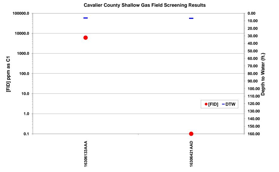
Figure 41. Shallow gas field screening results in Cavalier County. FID response [FID] in ppm as C1 is plotted on the logarithmic scale on the primary y-axis. Depth to water measurements are plotted on the secondary y-axis.
