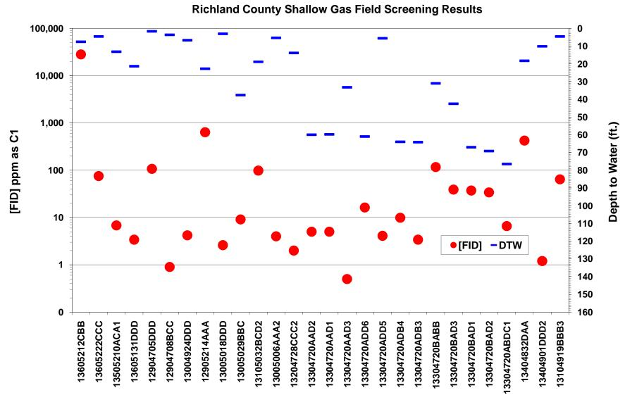
Figure 23. Shallow gas field screening results in Richland County. FID response [FID] in ppm as C1 is plotted on the logarithmic scale on the primary y-axis. Depth to water measurements are plotted on the secondary y-axis.
