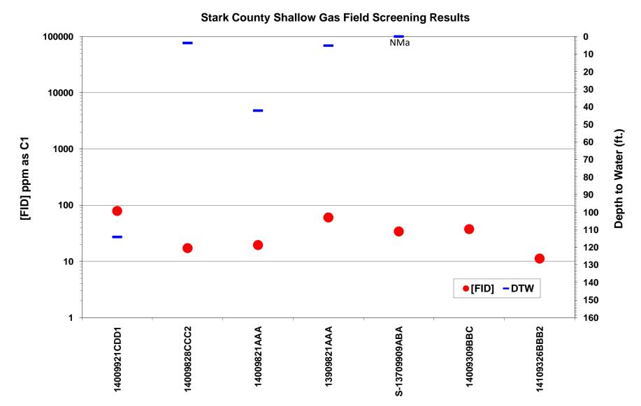
Figure 19. Shallow gas field screening results in Stark County. FID response [FID] in ppm as C1 is plotted on the logarithmic scale on the primary y-axis. Depth to water measurements are plotted on the secondary y-axis. NM = Not Measured. S = Stock Well. a = artesian well.
