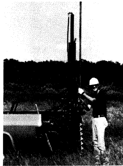
Figure 1. Former NDGS geologist John Graham, operating the Giddings soil probe.
