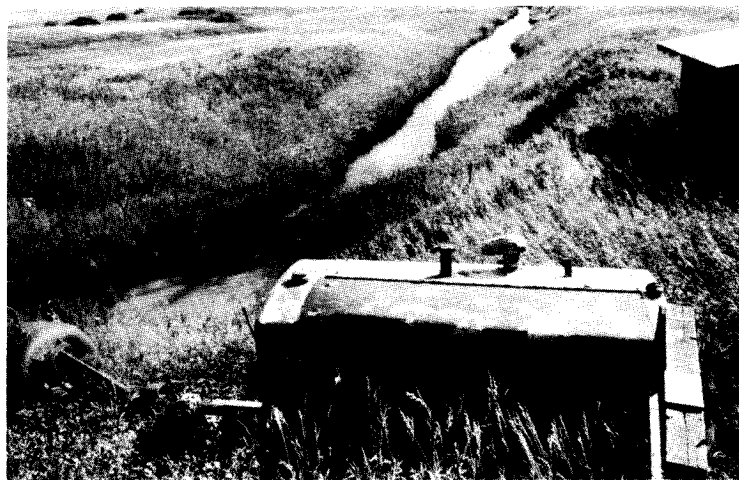
Figure 5. The Sodium Corporation of America's pump used to transfer brine from Miller Lake into their settling pond on North Lake, Divide County.
