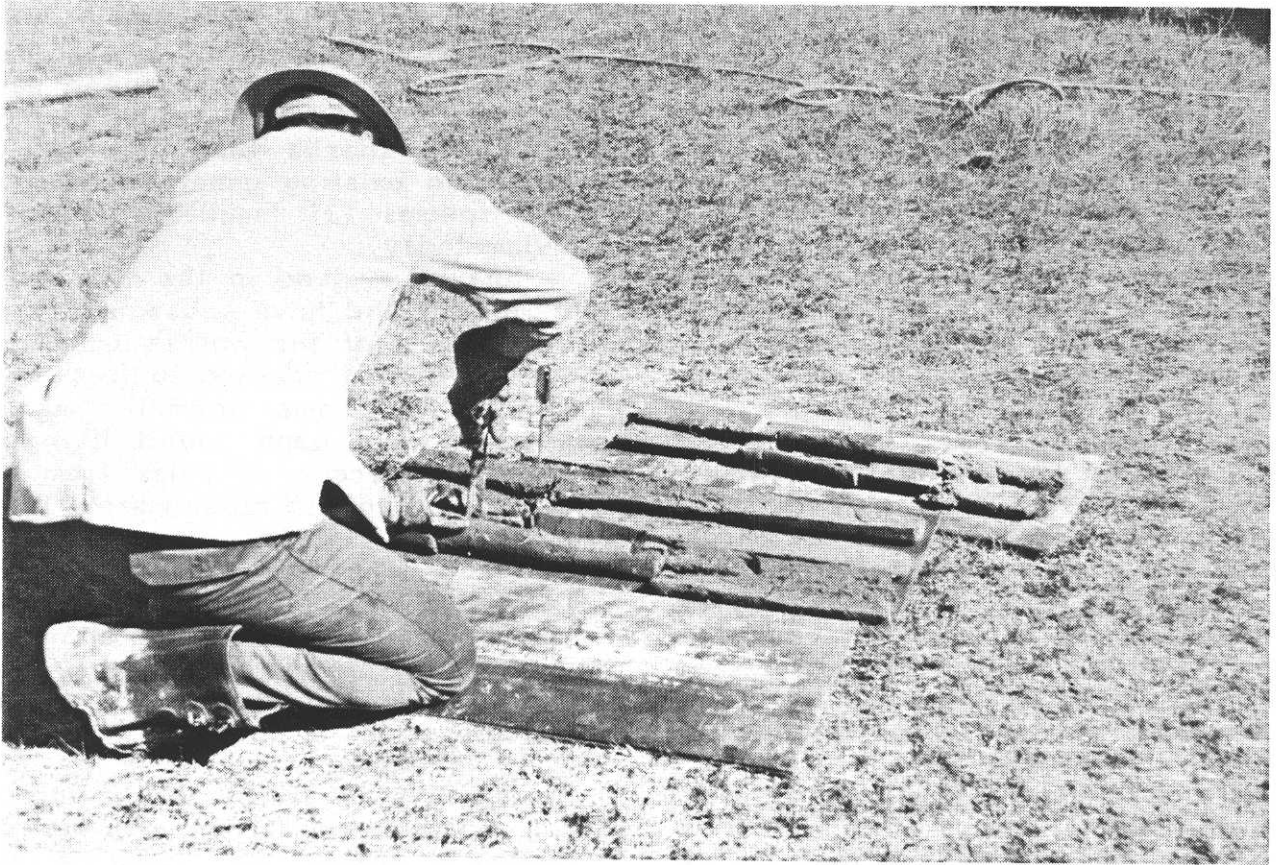
Figure 2. Test hole sample cores laid out for inspection. We obtained cores of the glacial sediment and lake sediment in the upper 25 feet in the area surrounding the lagoon. The undisturbed cores give us a better idea of the composition, consistency, texture, and permeability of the materials and help us determine whether the lagoon might be losing water through the ground.
