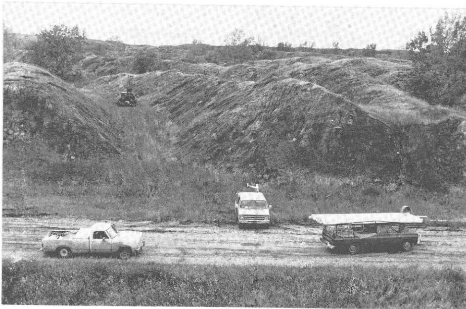
FIGURE 3 - AUGERING LYSIMETER BORING NO. 7 IN THE NOONAN MINE. ACCESS LIMITED TO LOCATIONS OF LYSIMETERS TO THE V'S OF THE SPOILS. NOTE THE STEEPNESS OF THE SPOILS AND THE SPARSE VEGETATION. THE GEOPHYSICAL VAN IS LOGGING PIEZOMETER TEST HOLE NO. 12.
