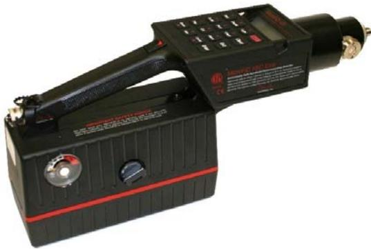
*Figure 2. Photovac portable Flame Ionization Detector (FID) used in this investigation.*
