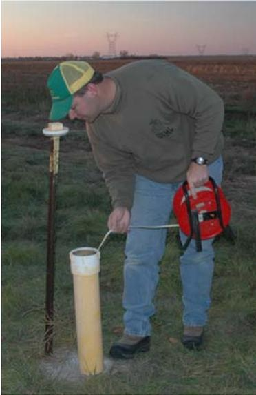
Depth to water measurements (in feet) were taken at each well field screened where a positive FID instrument response was recorded. A total depth of well measurement was also consecutively collected, when required, in order to identify individual wells within well nests that were not readily identifiable in the field. All ground-water level measurements were collected with an electronic well tape during field screening.
