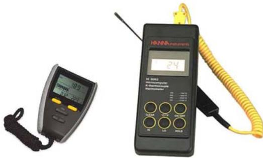
*Figure 6. Field instrumentation used for the collection of atmospheric pressure and temperature.*
