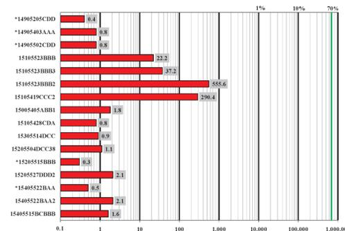
Figure 1. Graph depicting the relative relationship and absolute maximum values of flame-ionization detector (FID) instrument responses from selected wells in Grand Forks County. FID results for each well are presented in order of field screening occurrence from top to bottom. Values shown are those reported from the ground-water/air interface (GWI) (as CH<sub>4</sub> in ppm). The concentration of methane typical in commercial natural gas is highlighted by the vertical green line at 70%.
