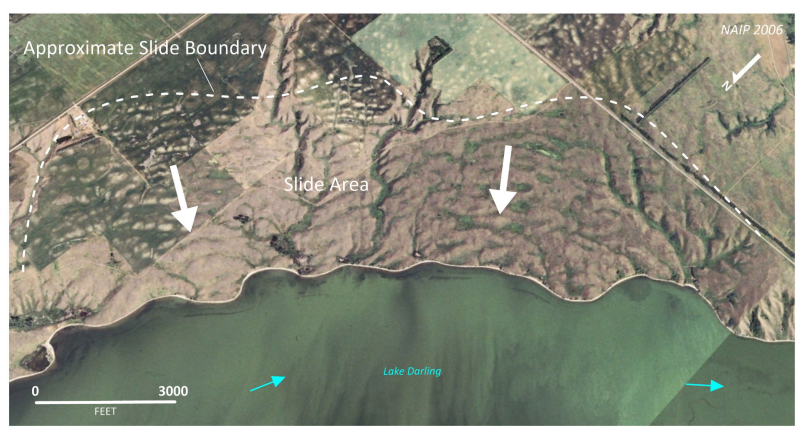
Qlsm Landslide area along the southeastern end of Lake Darling (not in map area) as an example of the jumbled topography and concentric lineation trends consistent with these types of landslides. Slides like these, resultant from deglaciation and meltwater flow, are quite large and best observed in LIDAR and aerial imagery. View is to the southeast.
