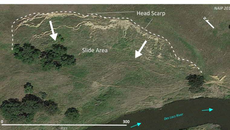
Qlsa Landslide area along the Des Lacs River Valley northwest of Burlington. This slump is along the valley wall and is likely the result of steep local slopes close to the fluctuating groundwater and river levels in this area. View is to the northeast.
