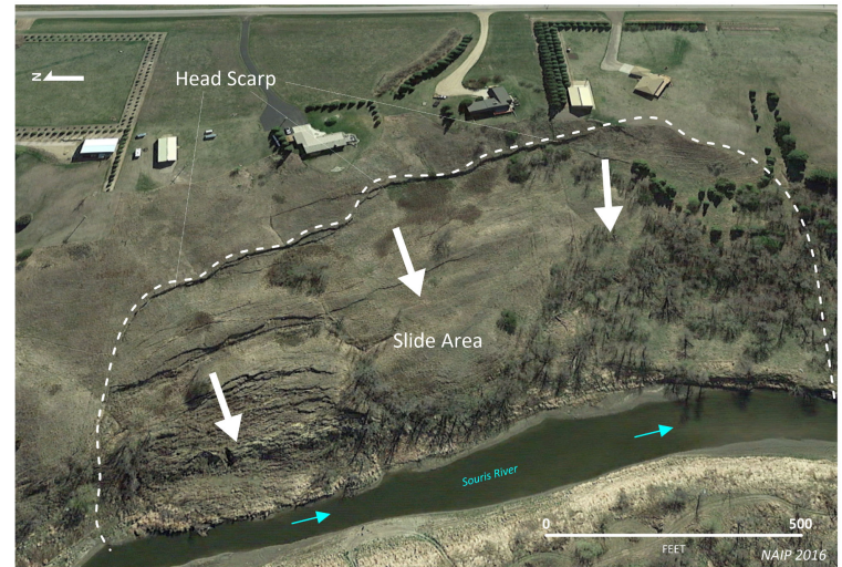
Qlsc Landslide area along the eastern bank of the Souris River just west of 55th Street in the southeastern part of the Souris River Valley. This slump has a head scarp near residential dwellings. A smaller more active area within the overall slide mass can be seen in the left foreground with parallel sets of tension fractures oriented perpendicular to downslope ground motion. View is towards the east.
