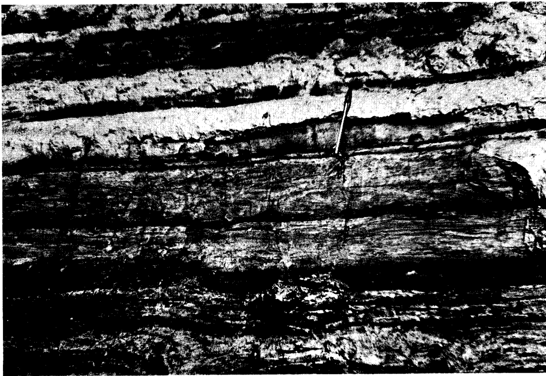
Figure 3. Close-up view of Figure 2. The stratification looks irregular when viewed at close range. Clay is dark colored, silt is light. Pen is 6 cm in length.
