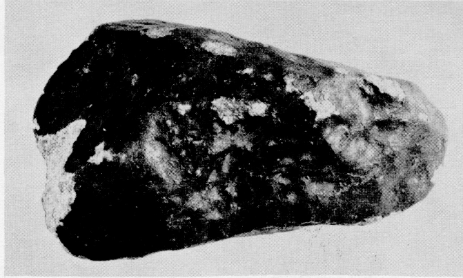
Figure 1. Richardton, North Dakota chondritic meteorite fragment showing irregular shape , pitted surface , black fusion crust and light gray stony interior . Natural size. (U.N.D. No. 2517)
