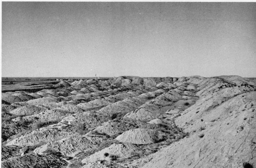
Figure 8 - Spoil piles of an abandoned dragline operation. Spoil pile in right foreground and continuing along right side of photo represents the first or outside cut. Piles to the left of initial pile are lower, representing succeeding cuts. Abandoned pit at far left. In the left background is town of Noonan. Location - Baukol, Noonan Pit in NW of Section 10, T. 162 N., R. 95 W., Divide County, North Dakota.
