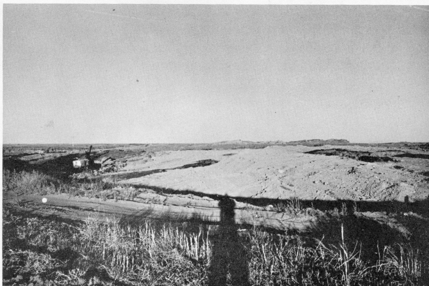
Figure 10 - View of active dozer and scraper operation taken from pitwall. Active pit with loading shovel in left foreground. Spoil piles in center and right foreground. Note gentle slope of spoil piles toward the pit and lack of vegetation. Location - Bonsness Mine in NW of Section 27, T. 162 N., R. 93 W., Burke County, North Dakota.
