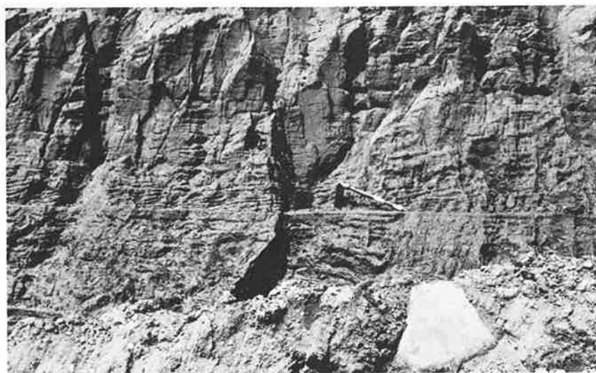
Figure 24. Two photos of a 55-foot excavation in southern Steele County (sec 19, T144N, R55W). Lake silt occurs between about 10 and 35 feet depth; surface elevations are about 1,180 feet. A bouldery till occurs in the bottom of the excavation. The silt is highly jointed, rather hard, and rhythmically banded. At 25-foot depth is a marked change in hardness that looks like an erosional break of some kind, perhaps a wave-cut surface. The silt beneath the break is considerably harder than that above. The upper photo shows the whole sequence; the lower shows a part of the silt unit with the ledge on the lower, harder silt.
