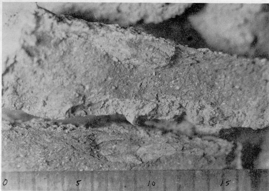
Figure 7. Drill cuttings from the Greenhorn Formation showing "white specks." Sample from test hole 2183, 134-52-6ccd; depth about 260 feet. Scale in millimeters.
