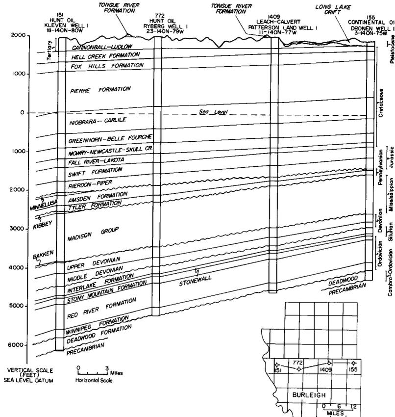
Figure 9. Burleigh County subsurface bedrock stratigraphic cross-section.
