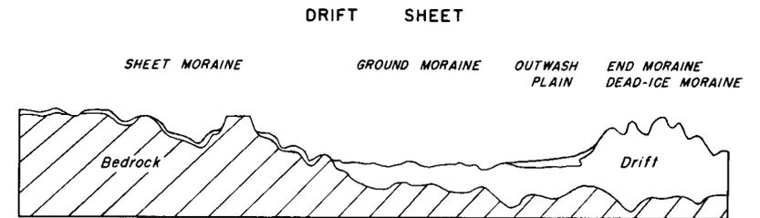
Figure 4. Diagrammatic profile and cross-section of a drift sheet.
