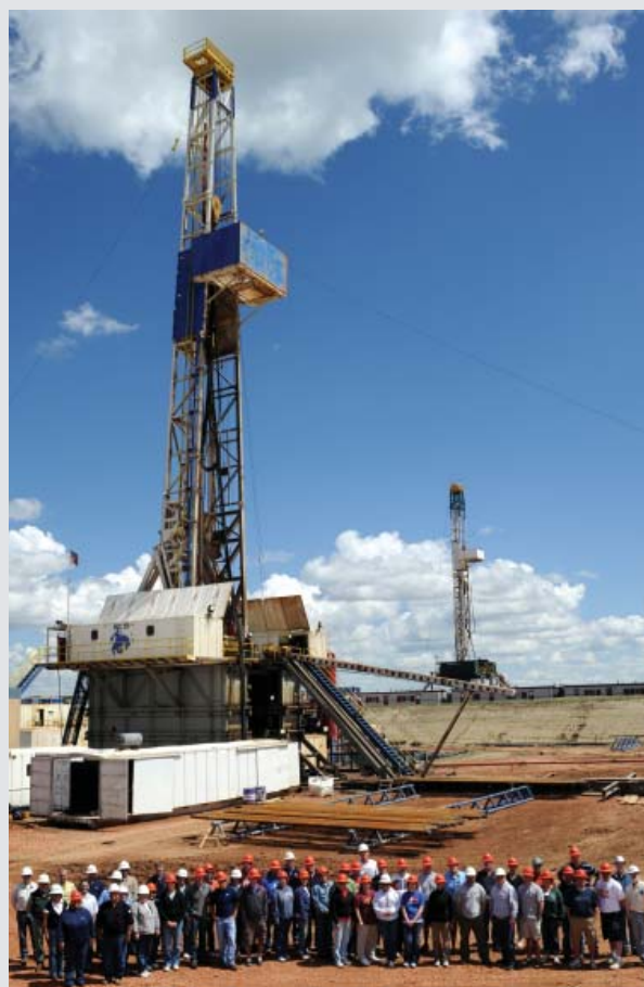
The group photo of the 2010 North Dakota Petroleum Council's Teacher Education Seminar provides a rare look at two drilling rigs in close proximity. A pipe wrangler or automated pipe handling system had just been deployed in the closest rig to bring a new section of drill pipe to the rig floor. Photo courtesy of the North Dakota Petroleum Council.
