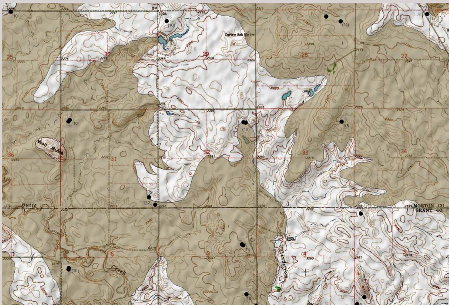
Figure 2. A portion of the Heart Butte coal map. The areas in brown indicate lignite reserves and the black dots are drill holes. The numbers adjacent to the drill holes are mineable coal thicknesses. If these numbers are in parentheses it signifies that it is a cumulative thickness of two beds.
