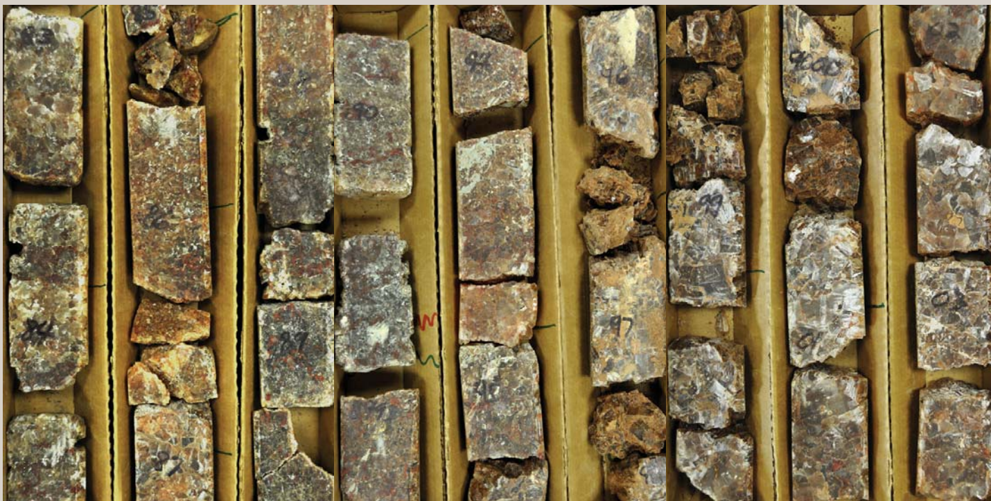
Figure 1. Twenty-one feet of salt core from a depth of 8,983 to 9,004 feet (going from 8,983 feet in the upper left to 9,004 feet in the lower right hand portion of the photograph) in the Texaco TXL storage well in central Burke County. Note the variable grain size, color, and clay content across this interval of the Esterhazy Member of the Prairie Formation.
