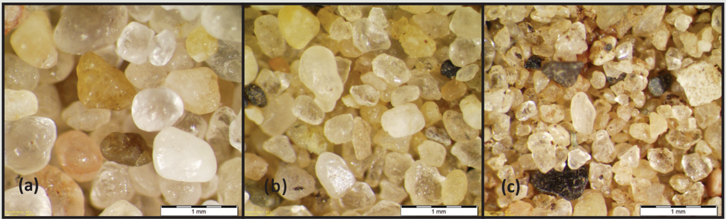
Figure 5. Photomicrographs of (a) an out-of-state proppant sand currently in use in the Williston Basin, (b) a North Dakota sand processed for use as a proppant, and (c) dune sand from Pembina County. All images are at 40x magnification.
