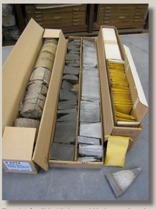
Figure 1. Left to Right: Whole core, slabbed core, and samples.
