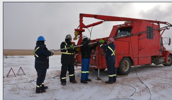
Figure 2. Logging crew connecting the tool to the slickline. From left to right: Mike Harden, WISCO, David Smith, WISCO, Jay Jamali, GoWell, and Kevin Hammer, WISCO.
