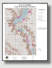
McDonald, M.R., 2015, Areas of landslides Carpio NE, ND Quadrangle: North Dakota Geological Survey 24K Map Series No. Crpo NE – I. Ten landslides were mapped within the Carpio NE Quad. The slides principally occur along the banks of Lake Darling and along the sides of the valleys (outside the floodplain) of the Souris and Des Lacs Rivers. These landslides occupy a total area of 385 acres with the largest covering 74 acres. Price: \$5.00 for traditional paper map and \$25 for 100k shape file CD.
