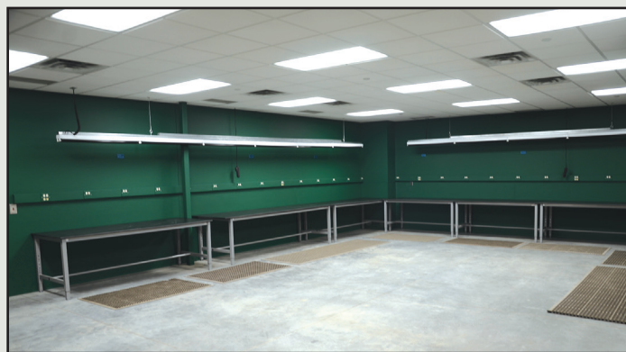
Figure 6. Blacklight lab on first floor of renovated building. Blacklights may be positioned using black control hanging from each panel of lights. Room painted green for ideal fluorescence when black lights are on.
