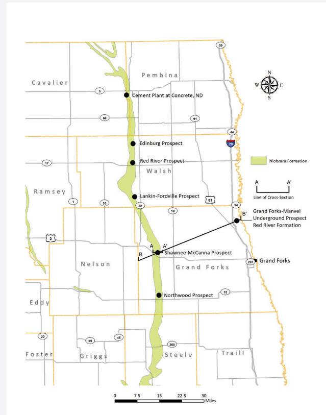
Figure 2. The Niobrara Formation subcrops in the shallow subsurface across a north-south trend in eastern North Dakota and outcrops in minor localities in northeastern North Dakota (modified from Bluemle, 1983). In northeastern North Dakota the formation is found at shallower depths than in the south making it a more favorable exploration target.
