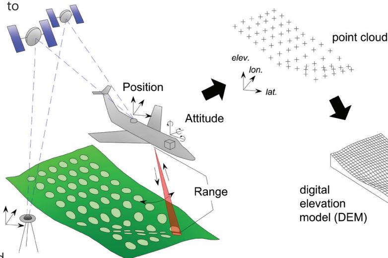
**FIGURE 3.** A General representation of airborne LiDAR being acquired and processed. Adapted from <https://historicmappingcongress.files.wordpress.com/2012/06/lidar.jpg> (Date retrieved July 7, 2016).
