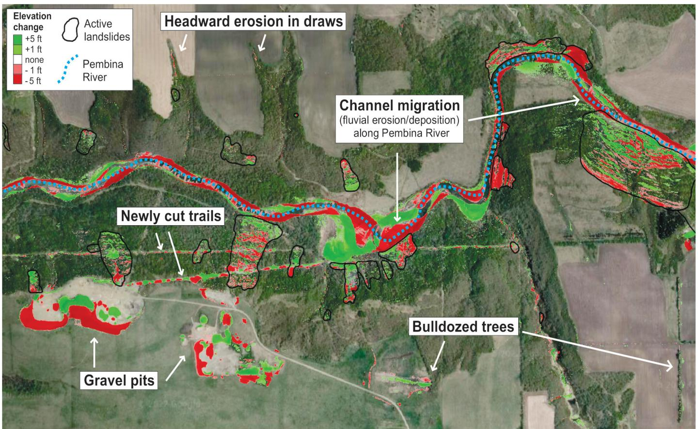
**FIGURE 11.** Differential elevation raster overlaid on aerial imagery of the Pembina River southwest of Walhalla, ND. Elevation changes (between 2008 and 2018) caused by landslides and many other sources are apparent.
