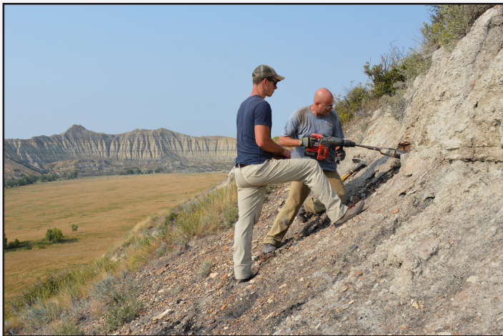
Figure 1. Survey geologists Levi Moxness (left) and Ned Kruger (right) use a battery-operated drill fitted with a soil auger bit to collect a coal sample in Slope County.
