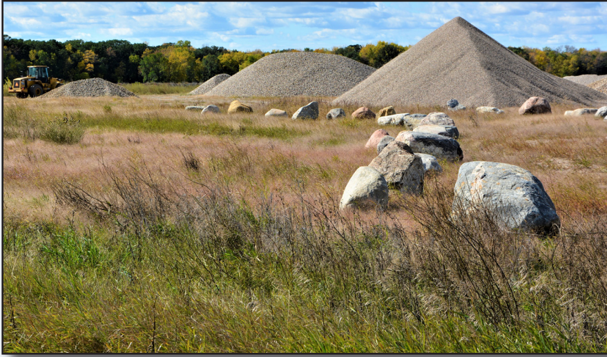
Figure 3. Sand and gravel pits like this one in McHenry County have been developed in Quaternary age glaciofluvial-deltaic sediment associated with the flow of glacial meltwater down the Souris River Valley. These pits produce a variety of materials from fine-grained sand to coarse gravel and large glacio fluvial meltwater boulders transported by glacial meltwater outbursts.
