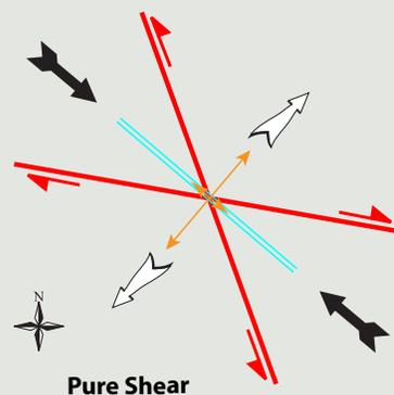
**Figure 2.** Geometry of structures formed during pure shear (A) at an active convergent plate boundary (northern Andes, South America) and simple shear (B) at an active transform plate boundary (San Andreas Fault, California). Modified from Sylvester, 1988.
