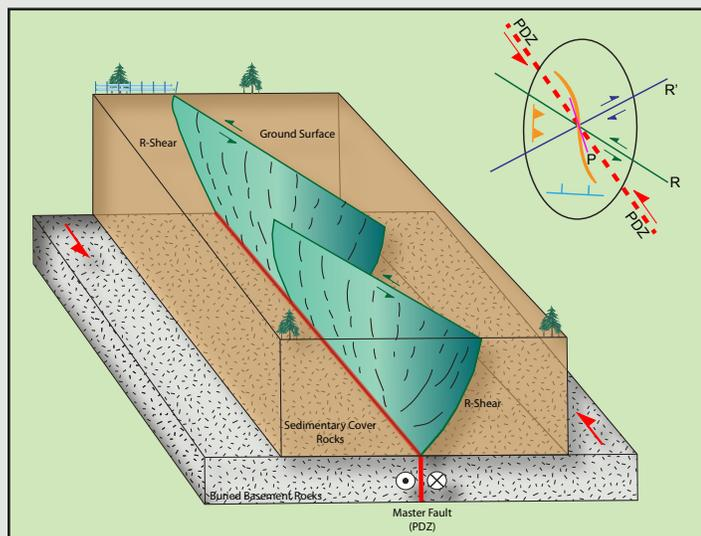
**Figure 4.** Block diagram of basement-rooted sinistral wrench fault and strain ellipse for comparison showing development of curvilinear and propeller-shaped R-shears in the sedimentary cover. See Figure 3 for abbreviations and strain ellipse designations.
