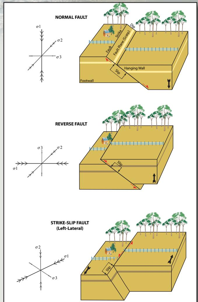
Figure 1. Block diagrams of dip-slip and strike-slip faults.  $\sigma =$  sigma.
