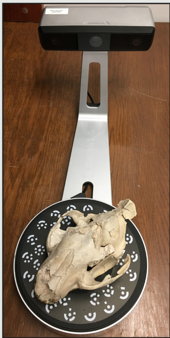
Figure 5. NDGS 3D scanner working to scan a specimen of Dinictis from the North Dakota State Fossil Collection.
