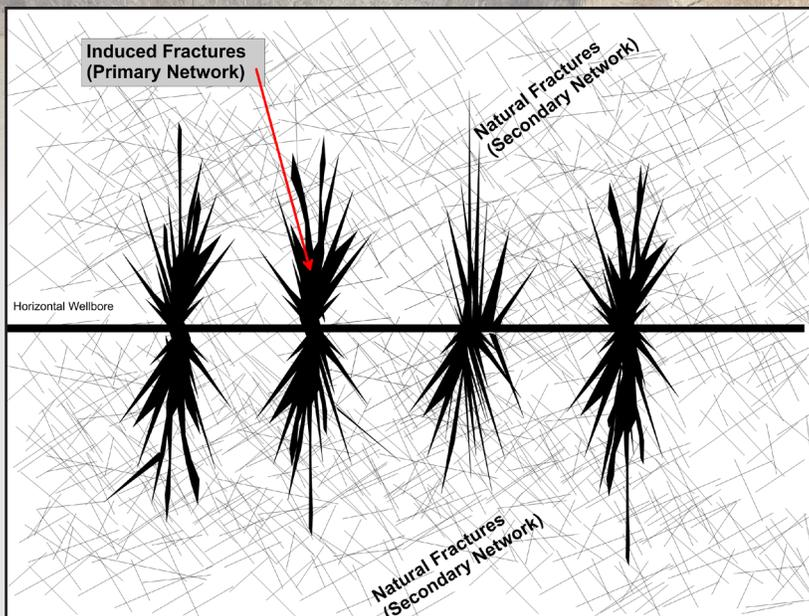
**Figure 1.** Conceptualization of natural and induced fracture networks in a reservoir rock with a horizontal wellbore.
