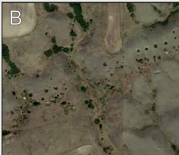
Figure 4. Sinkholes produced by collapsed underground lignite mines near Alkabo in Divide County. The larger sinkholes measure over 50 feet in diameter. The collapses are clearly expressed as circular depressions on bare-earth LiDAR imagery (A) and visible to varying degrees on Google satellite imagery (B).
