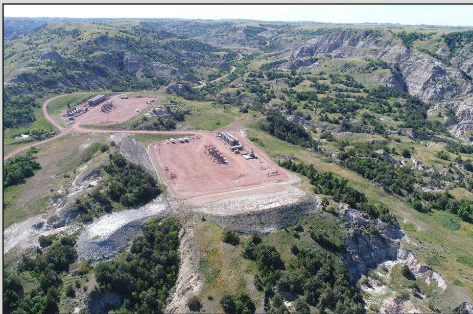
Figure 1. A drone photograph of a two-pad well site situated in the Little Missouri River badlands in Dunn County. Everything to the right (north) of the pads to the base of the cliff face is comprised of old landslides.
