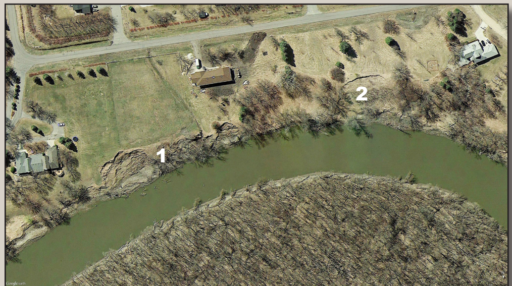
Figure 3. A series of landslides along 76th Avenue South in Fargo. One of the disturbed areas (1) extends for 500 feet and is up to 100 feet wide. The scarp of another landslide (120 x 160 feet in area) is visible midway between the two homes on the right (2). Nine homes had to be abandoned in this area due to slope stability problems including the home situated between 1 and 2. Photograph from GoogleEarth dated April 2014, looking south/southwest.
