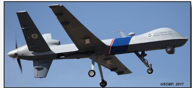
Figure 4. An MQ-9 Predator B Drone (Reaper), manufactured by General Atomics Aeronautical Systems. This is one of two Reapers operated by the U.S. Customs and Border Protection in support of the mission to secure the northern U.S. border. These drones have also supported flood-fighting efforts in the Red River Valley (USCBP, 2017).
