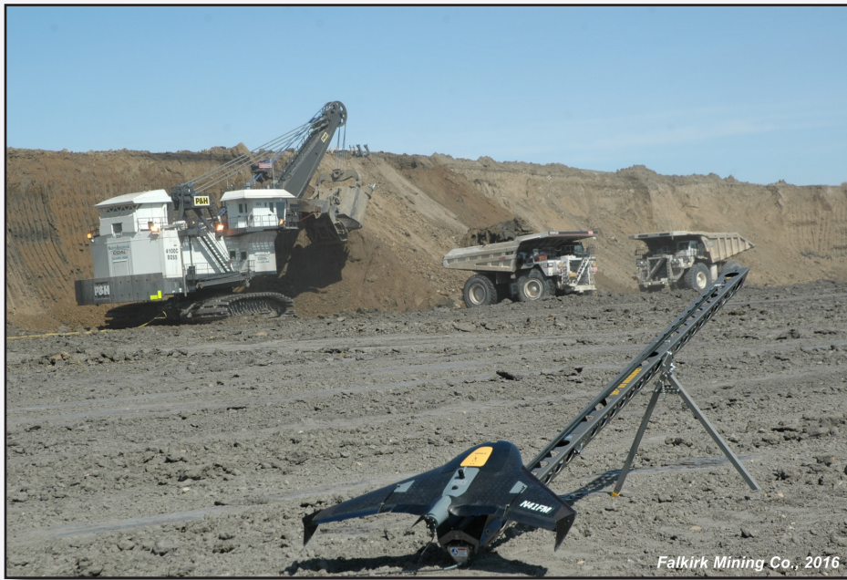
Figure 7. Technicians at the Falkirk Mine in central North Dakota have been using the Trimble UX5 drone to optimize mining operations since the fall of 2015.
