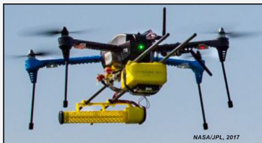
Figure 5. NASA JPL's OPLS sensor onboard this small drone can detect methane in concentrations in the parts per billion (ppb) range (about equal to one drop of water in an Olympic size pool) and could be an aid to future oil and gas pipeline inspections and surveys.
